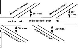
Back-draft damper kits (Part No. 3391910) are available from your Whirlpool dealer and should be installed in each dryer's exhaust duct to prevent exhausted air from returning into the dryers and to keep the exhaust balance within the main exhaust duct. Unobstructed air openings are required.
